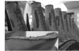
Erosion on HPT rotor blades, [5]
